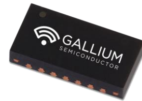
14 Pin 6x3 mm DFN Package
