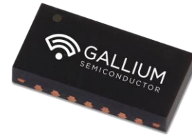
14 Pin 6x3 mm DFN Package
